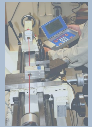
Microgage 2D Transparent Receiver shown on lathe alignment
