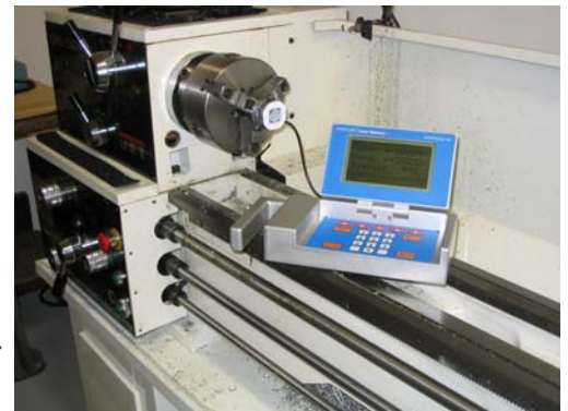
The Microgage Display is capturing readings from the 2D Disk Receiver
